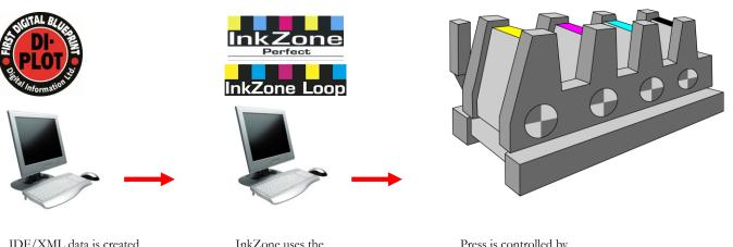
JDF/XML data is created out of CIP3 or 1-Bit TIFF Bitmap data
