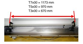
Add the tension roller and verify whether all three rollers can rotate smoothly.
