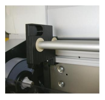
First, tighten firmly the left "side holder" to the base profile. Position it at the end of the profile.
