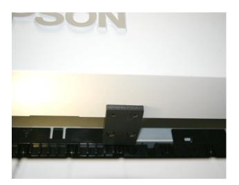
The picture displays a correct positioned plate. The paper can exit without the risk of a paper jam.
