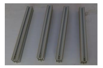
Frist, insert 4 slot nuts M8 into each base profile Nr.1. Then mount profile Nr.2.
