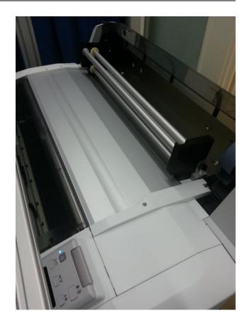
Finally, tight firmly the two M4 screws to mount the "paper entry guide" to the printer.
