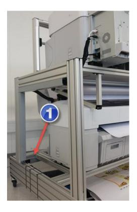
Take the cables from the lower camera system into the horizontal profile (1).
