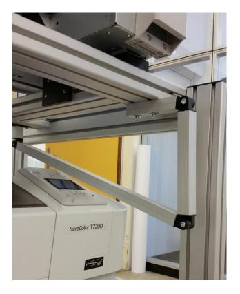
Position the centre line of the 25mm profile 65 mm from the right profile edge.
