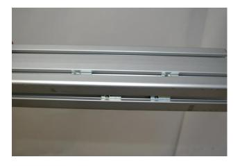
Insert two slot nuts M8 into the upper side of the cross section profile (top right cross section profile)
