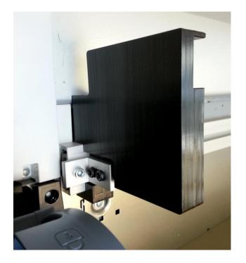
Add the slot nut M5 into 15x40 profile and mount the right side holder to it.
