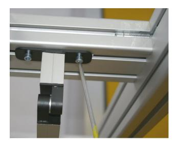
Add two slot nuts M5 (full size) and mount the other side with the M5 x 35 like shown.
