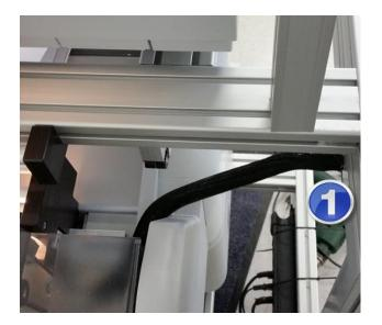
Put all cables from the top printer into the horizontal profile.
