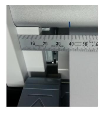
The distance between the roll holder and the mark (paper entry) should be approx. 4 mm.
