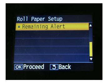
For the front printer only: Set the "Remaining Alert" = 10 m
