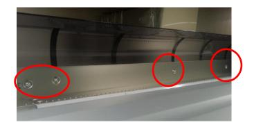
Now bend the back cover on the right side a bit backward to access the screw which mounts the paper roll holder guide.
