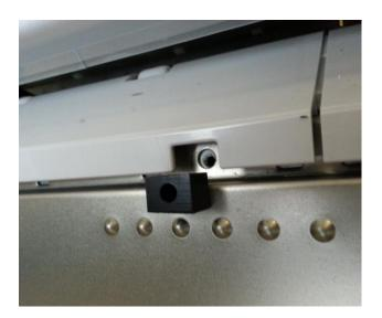
Put the POM part into the aperture as shown.
