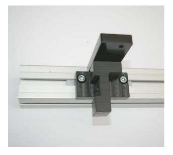
Use the M3 screw to bolt the LED to the camera holder. The angle is approx. 45 degree.
