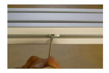
Insert two slot nuts M8 into the upper side of the cross section profile (top left cross section profile)
