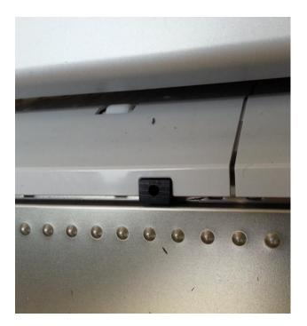
Use the M4 x25 screws to mount the profile to the printer.
