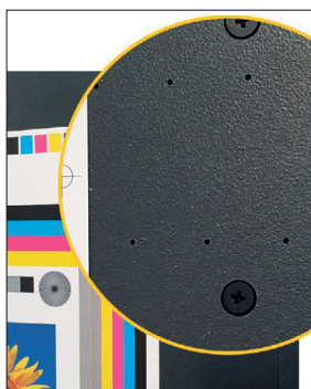
Two rows of vacuum holes for substrate fixation.
