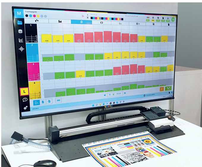
InkZone Move visualizes all color measurements of the Myiro spectrophotometer in real time.
