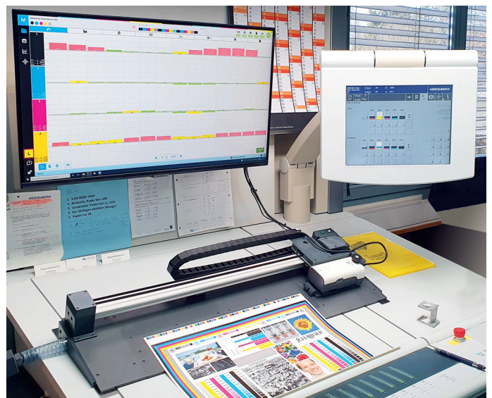
Heidelberg Speedmaster 52 offset press with InkZone ColorTrail and the Myiro spectrophotometer.
