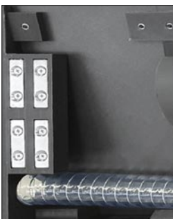
Back side of the vacuum system with magnetic fixation.
