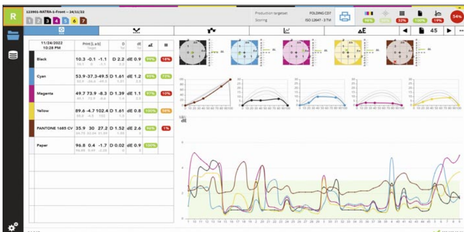
InkZone Report showing TVI over a press run.
