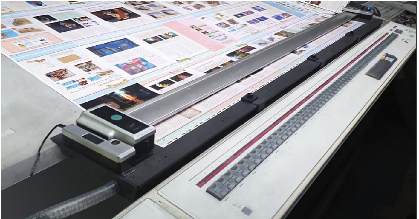
InkZone Vacuum in operation on a Manroland R900 XXL console.
