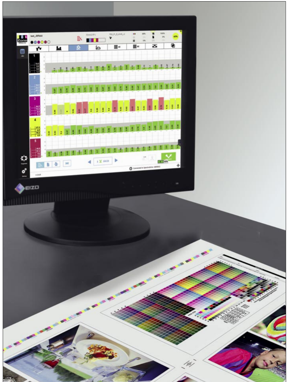
InkZone Move shows color results for every ink key immediately after scan.
