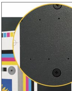
Two rows of vacuum holes for substrate fixation.
