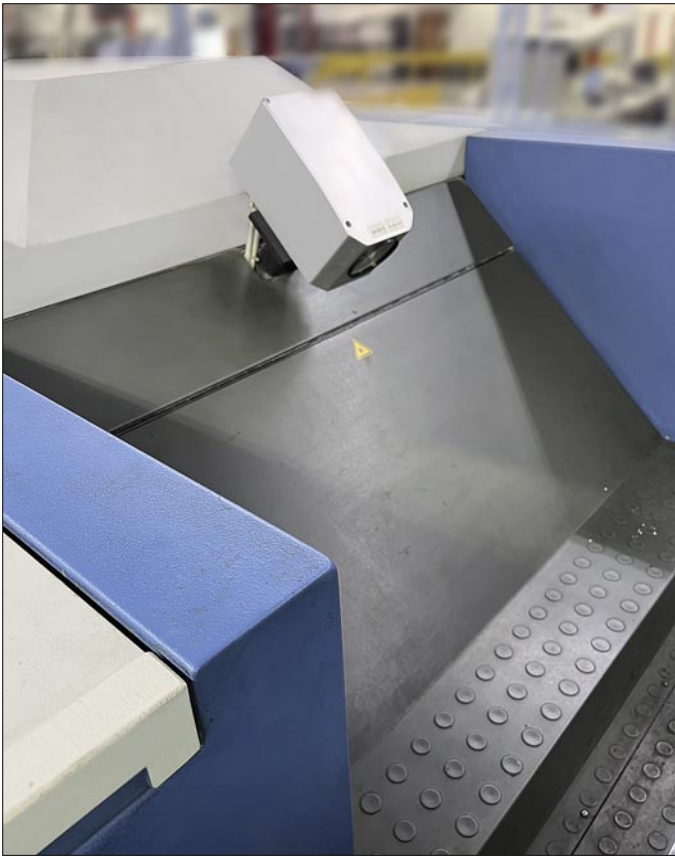
State of the art color bar image caption device for inline density measuring.
