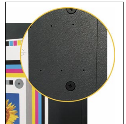
The double-row vacuum hole system.
