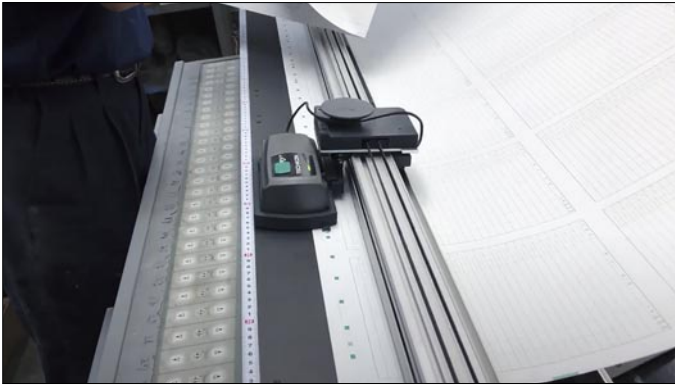
Techkon's SpectroJet spectrophotometer mounted on the InkZone ColorTrail automated track.
