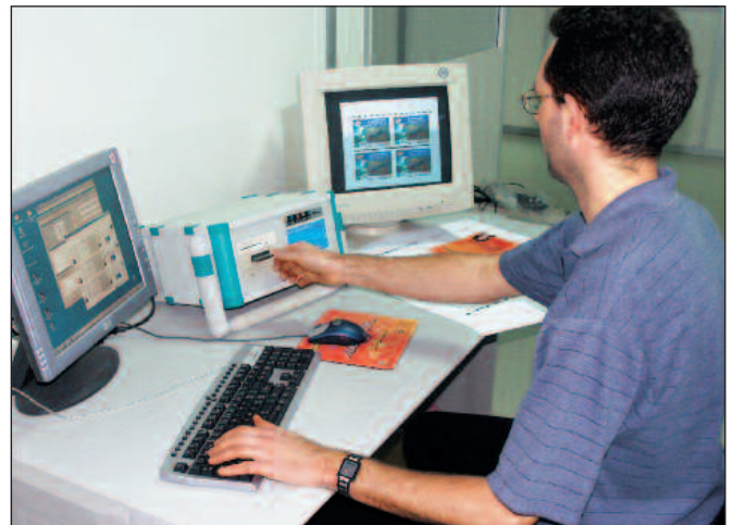
InkZone Box (centre) writes the ink zone preset data in all familiar printing machine formats to the corresponding data carriers. To the left of the picture is the user interface to the DI-Plot form proof software; the screen on the right shows a preview of the imposed print form.
