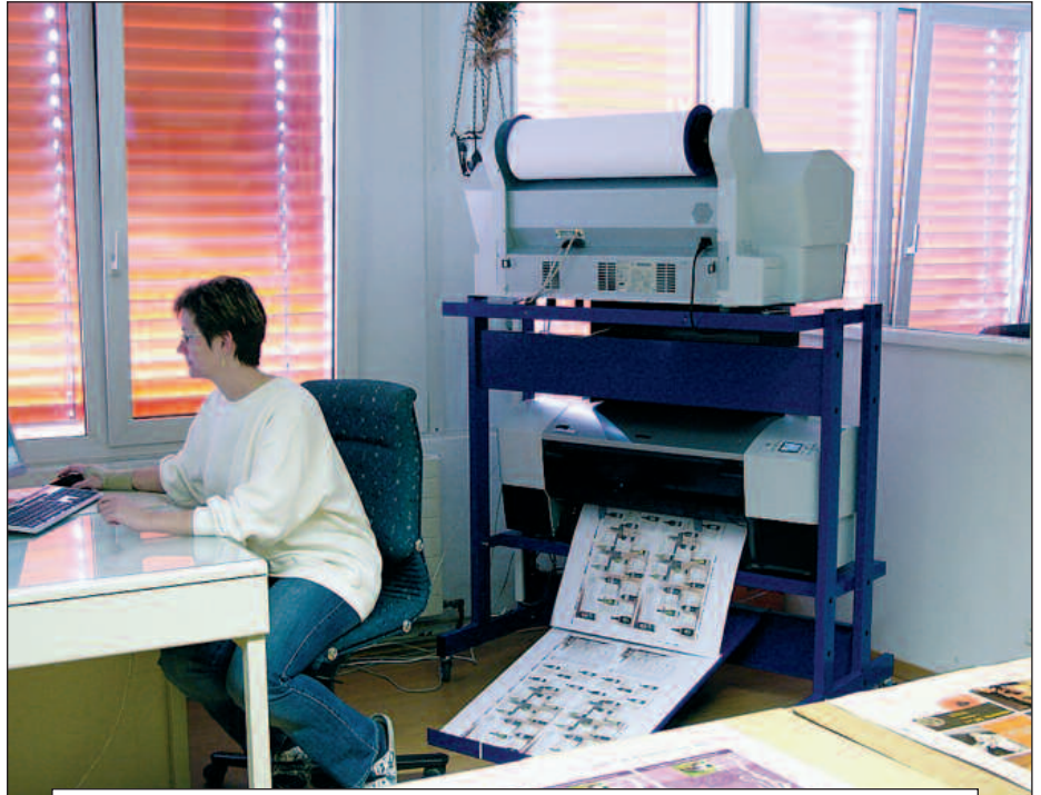
Preproofer 740 runs at up to 16 double-sided printed formproofs per hour.
